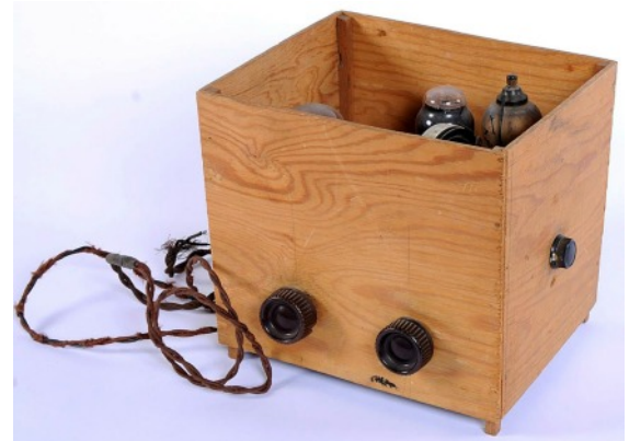
3 valve home constructed illegal radio receiver in a wooden box.
