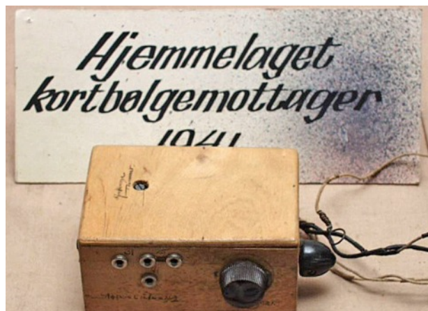
Home build illegal short wave radio receiver housed in a small wooden box.
