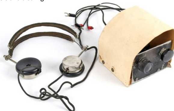
Home made radio receiver used in the Haugesund area, probably powered by an accumulator and HT batteries.
