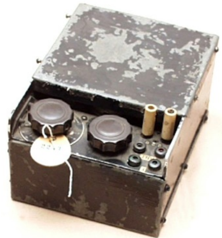
Miniature illegal short wave radio receiver (9x13x16cm).
