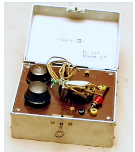
Battery powered illegal receiver concealed in a metal cash box.
