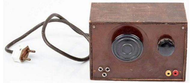
Illegal miniature home made mains powered radio receiver in a wooden box.
