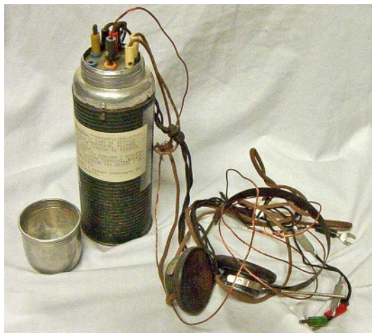
This thermos flask radio receiver was constructed by Eystein Schejetne in 1943 and used during the rest of World War 2. It was powered by 1.5V LT and 60V HT batteries, the latter by connecting a number of 4.5V flashlight batteries in series.
