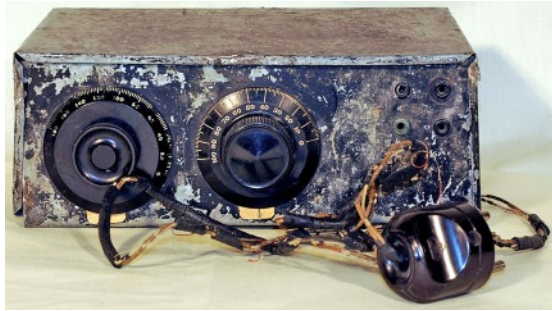
Mains powered illegal radio receiver build into a small tin box.
