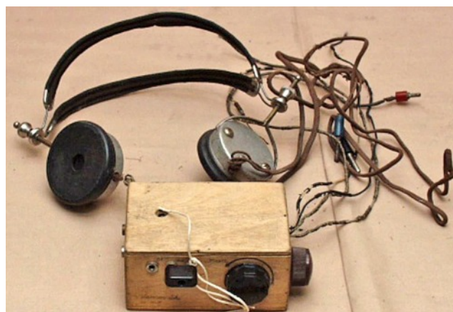
Illegal short wave receiver most likely build by the same maker of the radio shown on the left.
